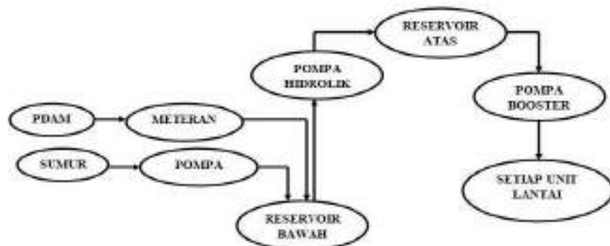
Bagan 12. Skema Distribusi Air sistemDown Feed
