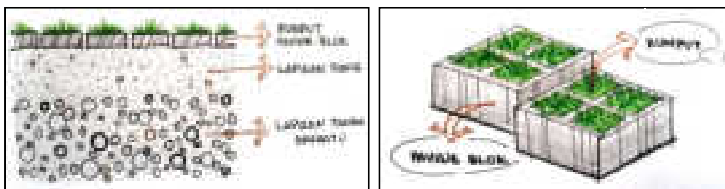
Gambar 5. 10 perkerasan paving blok
