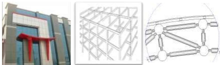
Gambar 5.17 super struktur (aluminium komposit, rangka kaku, space frame) ( sumber : https://www.arsitur.com )
