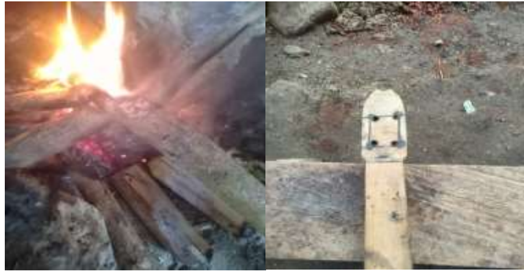
Gambar 4.25: proses melubangi Bradan Fatin Sumber: Dok.Alexis 02/04/2024
