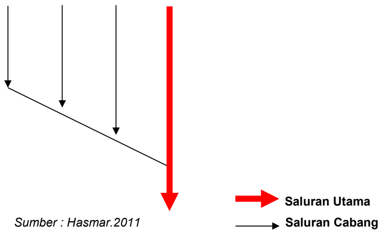
Gambar 2.3 Jaringan Drainase Grid Iron
