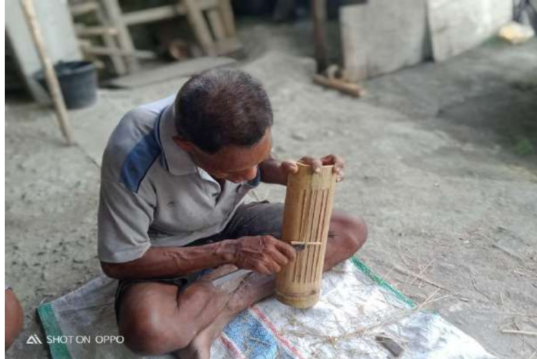
Gambar 4.22. Proses mengikis kulit bambu Dok. Johan November 2022
